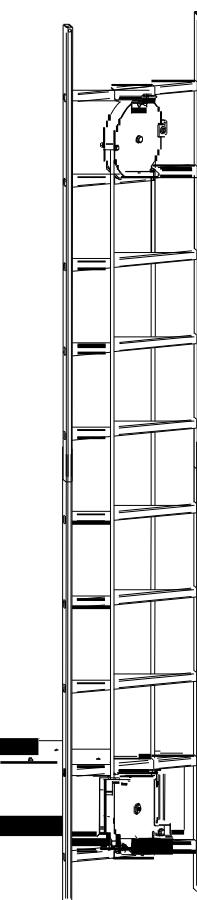
The ascending and descending climbing assistance is a useful element for medium-height wind turbines and for those not fitted with an industrial hoist. This device facilitates the maintenance technician's work, preventing injury to the knees, arms and feet.
